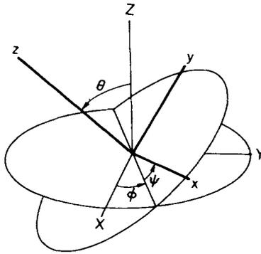
Fig. 1. The three Euler angles  $\theta$ ,  $\phi$ , and  $\psi$ . These specify the orientation of the local system of axes  $x(s)$ ,  $y(s)$ ,  $z(s)$ , defined at each distance  $s$  along the rod, relative to fixed space axes  $X$ ,  $Y$ ,  $Z$ . The local  $z(s)$  axis points in the tangent direction to the central axis of the rod.
